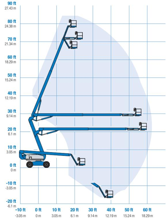
\* The metric equivalent of working height adds 2 m to platform height. U.S. adds 6 ft to platform height.
